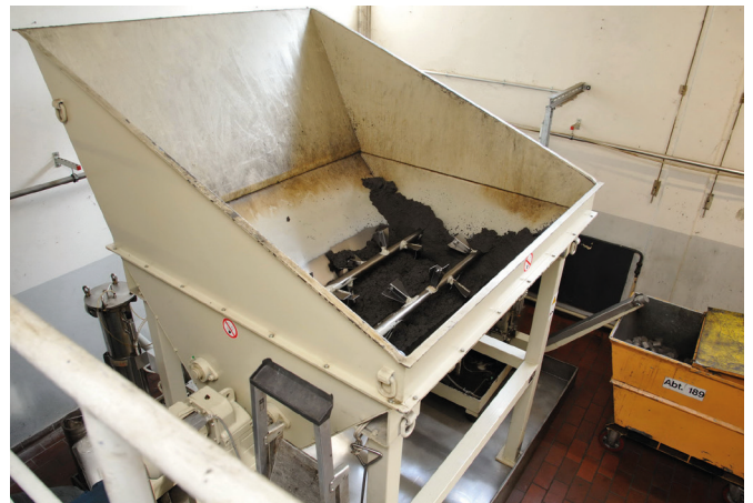
The grinding sludge from steel machining is transported in 0.4 cubic meter containers (upper image: in the Thyrnau plant / lower image: in Plant 1 in Passau) to the briquette press and filled into the machine's supply hopper with a forklift truck.
