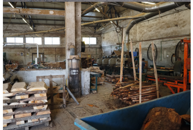
The path to completed Wooden pallets at Košcal starts from tree trunks, which are purchased as raw material. These are cut with band saws and multi-blade saws in the production area and then, mainly automatically, put together in the assembly area.
