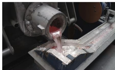
When the charging is completed, the liquid material is mostly cast into ingots and transported in this form to customers from the most varied branches.
