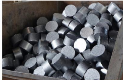
The designed set-up of the system as well as the high hydraulic pressing power of 2500 kg/cm 2 are decisive for the high quality of the briquettes created.
