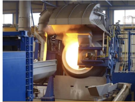
The modern tilting rotary furnace at MT Comax is fed with chips, which have been briquetted. The main reason: the yield of the briquettes is on average about five per cent higher.
